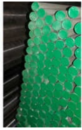
416 Magnetic Stainless Steel Round Bar
