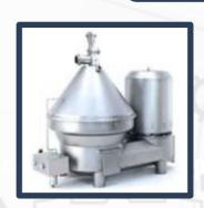
Cream Separator is machine used for separating and removing cream from whole milk; The separator consists of a centrifuge in the form of a rapidly revolving bowl containing a set of disks mounted on a spindle situated underneath the milk supply tank.
