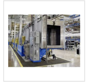
Industrial Spray Pre Treatment Line
