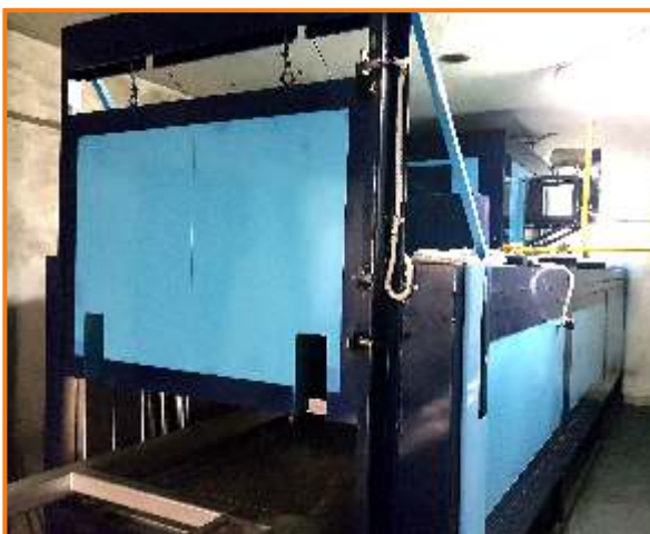
WOOD GRAIN SUBLIMATION MACHINE (for Aluminum section and steel doors etc)
