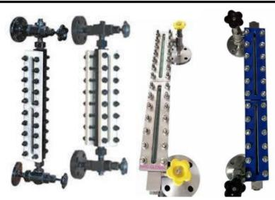
NRG offers a series of level indicators. Designed to measures the level of liquid in reactor tanks. The reflex level gauge is used for the measurement of liquid level for high pressure or high temperature or toxic liquid storage tanks. The reflex level gauge has a single prism glass mounted on one side of the chamber and uses the basic optical principles of light reflection to upgrade the expression of the liquid level in the process tank.
