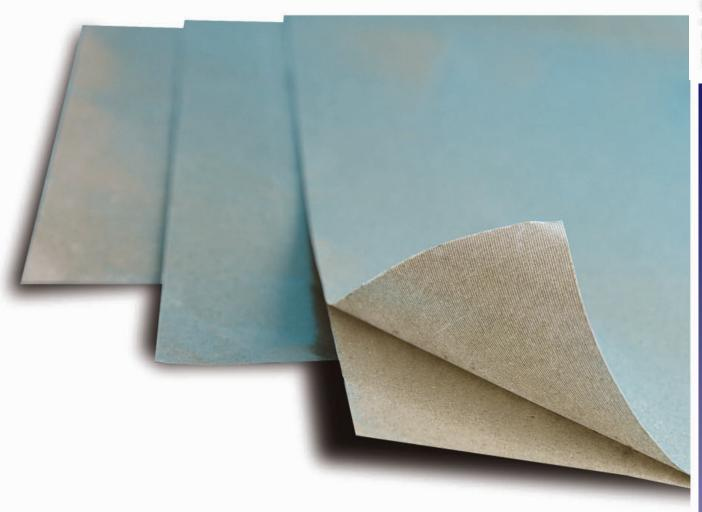
**Ruby Mica® Glass / Mica Folium** is a lamination of uncalcined phlogopite mica paper with a glass cloth. High thermal-grade silicone resin is used as a binder. This highly-flexible material can easily withstand temperatures to the tune of 950° C.
