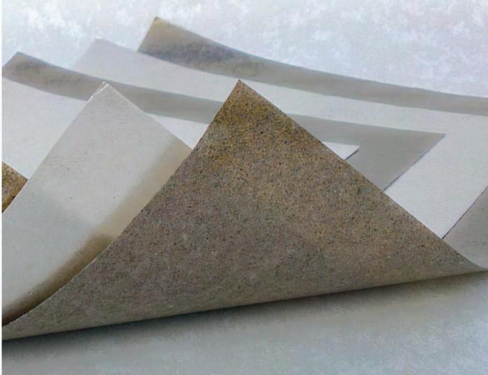
**Ruby Mica® Flexible Mica Laminate** is made by combining uncalcined muscovite or phlogopite mica paper with an inorganic silicone resin binder under specific heat and pressure.
