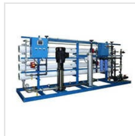
Industrial RO Plant
