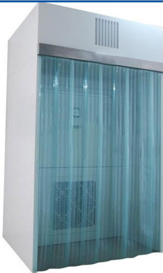
The weighing room is one kind of clean equipment which used in micro-organism research, pharmacy and scientific experimentation, it can supply the single and multi-way airflow, and clean air (HEPA AIR) will be circulated in the working area, the other part will be exhaust outside, it can make the working area negative pressure to prohibit cross population, it can guarantee the working area with high clean grade.
