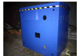
Blower Acoustic Enclosure
