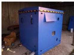
Blower Acoustic Enclosure
