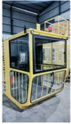
EOT Crane Operated Cabin
