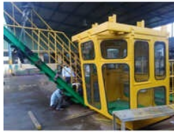
MS EOT Crane Operated Cabin
