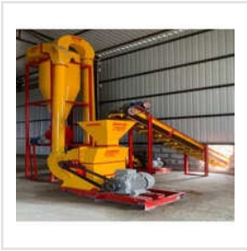
Biomass Hammer Mill
