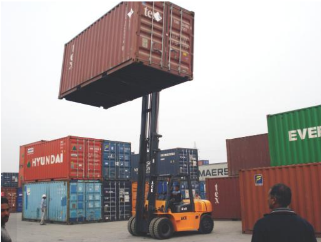
Model AF80D (Empty Container Handler) Robust design to handle 3 high stacking (6 mtr lift height) Fitted with wide carriage and 2400 mm long forks for stability
