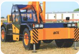
3 OUTRIGGERS Front Outriggers for added safety during high lift operations.
