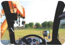
4 INCREASED VISIBILITY Bigger size front windscreen and re-routing of hoses provide much better front visibility.
