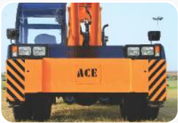
2 GROUND CLEARANCE High ground clearance of 300mm for easier rough terrain operation.
