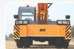
2 GROUND CLEARANCE High ground clearance of 300mm for easier rough terrain operation.
