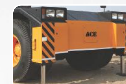
3 OUTRIGGERS Front Outriggers for added safety during high lift operations.
