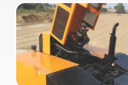
5 EASY MAINTENANCE The engine is easily accessible for daily maintenance checks including battery, air filter, oil dipstick and cooling system
