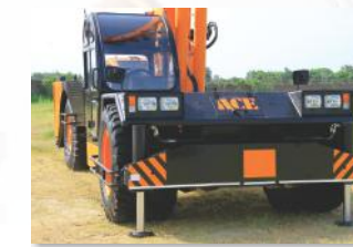
9 OUT TRIGGERS Front outriggers are provided as standard fitment for added safety during high lift operations.
