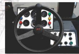
2 STEERING WHEEL & CONTROLS Steering wheel is provided as a standard feature, which along with ergonomically placed operator console and instrument cluster ensures ease of operation.
