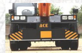
6 GROUND CLEARANCE Ground clearance of 300mm facilitates easier rough terrain operations.
