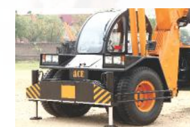
10 FRONT OUTRIGGERS Front Outriggers are provided as standard fitment for added safety during high lift operations.
