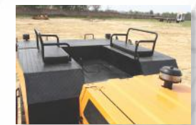
5 REAR DECK Spacious & well laid out rear deck for storing lifting tackles etc. and provides ample space for slingers/helpers.
