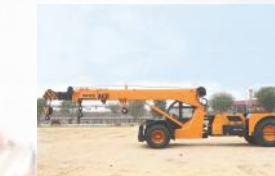
8 OPTIMIZED KINEMATICS AND LOW C.G. SX170 crane has been designed with low Center of Gravity (C.G.) providing best in class stability and operational safety
