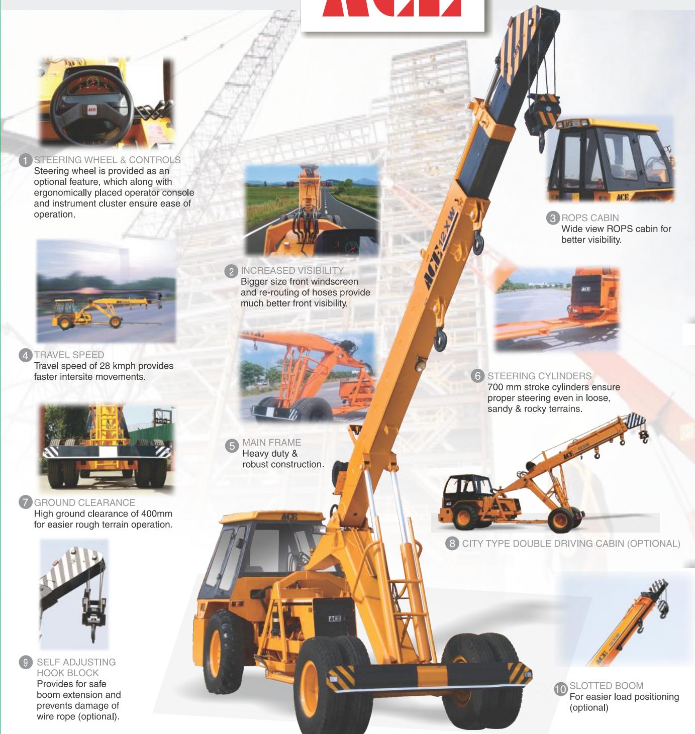
ACE 12 XW Model Crane fitted with 3 part boom (11.25 mtrs. height)
