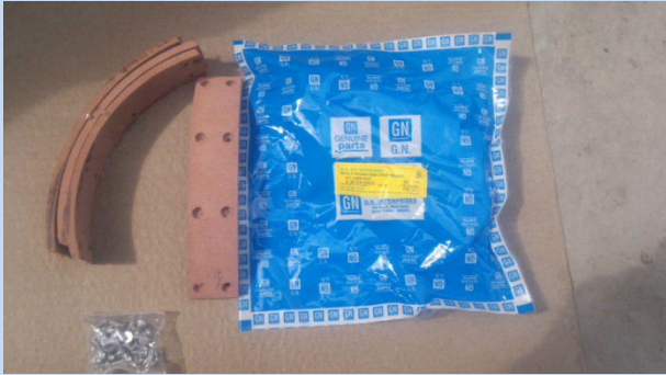
BRAKELINING SET WITH RIVETS
