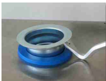
Push the filter holder out by a tool gradually step by step
