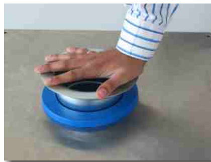
Press the filter holder evenly onto the cartridge
