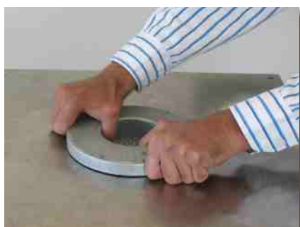
Pull the filter cartridge with hand gradually step by step
