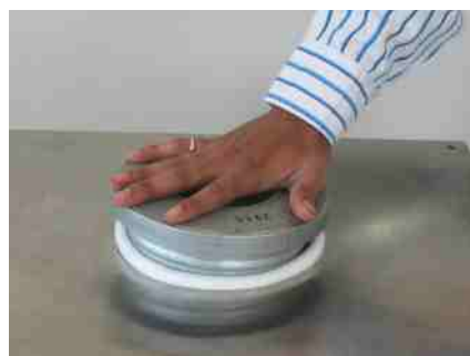
Press the filter cartridge evenly into the snap cuff
