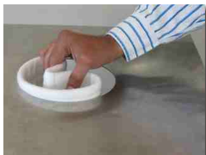
Place the snap cuff inside the mounting plate hole
