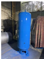
300L Air Receiver Tank
