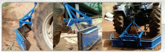
Scrapper Fitted To Tractor For Easy Use On Cattle Farm
