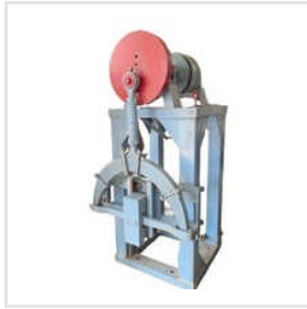
35 Kg 14 Inch Power Hammer Machine
