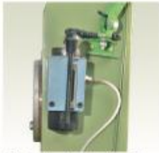
Centralized Lubrication Pump
