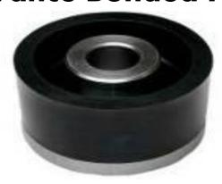
The **SUDARSHAN ADVANCE BONDED PISTON** is constructed of Nitrile rubber bonded to a well designed metal hub. The oil resistant rubber is designed to provide optimum performance in oil based or water based mud and high drilling pressures. The bonded construction resists extrusion under pressure and restricts movement to reduce the build-up of heat.
