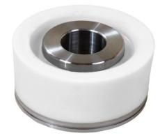
The **SUDARSHAN POWER PERFORMANCE BONDED PISTON** manufactured from special grade urethanes compound with dual hardness that provides resistance to water, oil and synthetic based drilling fluids ,these piston that is highly resistant to abrasion and tear. The bonded construction resists extrusion under pressure and restricts movement to reduce the build-up of heat.
