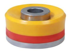
The **Sudarshan Extreme Pistons** are manufactured from urethanes compound with dual hardness that provides resistance to water, oil and synthetic based drilling fluids. The compound also provides superior resistance to tear, abrasion and extrusion and as the name suggests it is capable of operating in extreme conditions of fluid temperatures up to 300°F (150°C) and high pressure UPTO 7500 PSI.
