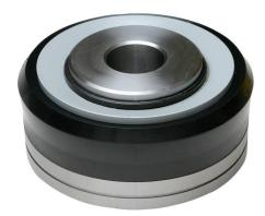
The **SUDARSHAN PINNACLE ASSEMBLED PISTON** is designed for use in the most demanding applications. The replaceable seal element is manufactured from a specially formulated elastomeric compound designed to be resistant to most chemical fluid found in the drilling industry today. These pistons can also be used in conditions where elevated temperatures can be problematic to other types of pistons in the market.
