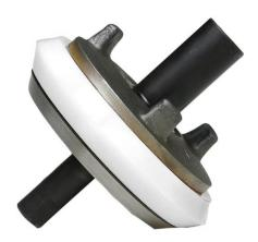
**SUDARSHAN STEM GUIDED VALVE ASSEMBLY (HTHP)** consisting of Valve Seat, Valve Body, & Valve Insert are available for different API valve pot sizes. Special care is taken for the dimensional matching of valve seat and valve body working angles for ensuring very high life even under extreme working conditions. Valve Insert is made out of **special grade urethane** material capable of operating in fluid temperatures of up to 300°F.
