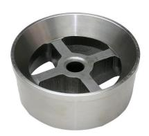
**SUDARSHAN STEM GUIDED VALVE ASSEMBLY** consisting of Valve Seat, Valve Body, & Valve Insert are available for different API valve pot sizes. Special care is taken for the dimensional matching of valve seat and valve body working angles for ensuring very high life even under extreme working conditions. Valve Insert is made out of high quality polyurethane material capable of operating in fluid temperatures of up to 220°F.
