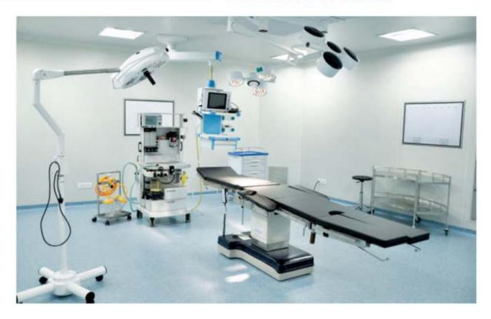
With the stand alone steel support or wall - mounted system Theatre has been built to suit many modern operation theatre applications. The wall panel is made of top class Electro Galvanized Steel with "no joint" finish after installation.
