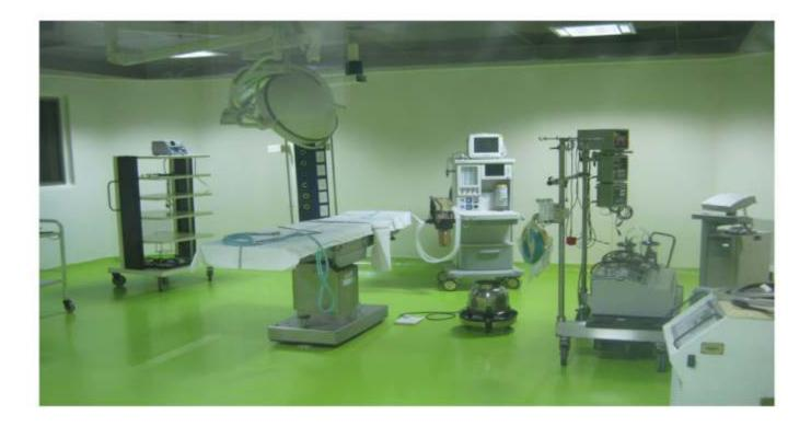
Flooring seamless with perfectly curved flash-covings, resistance to mechanical stresses and dynamic loads and having ESD/ EMI (conductive) protection characteristics, 2 mm thick, washable.
