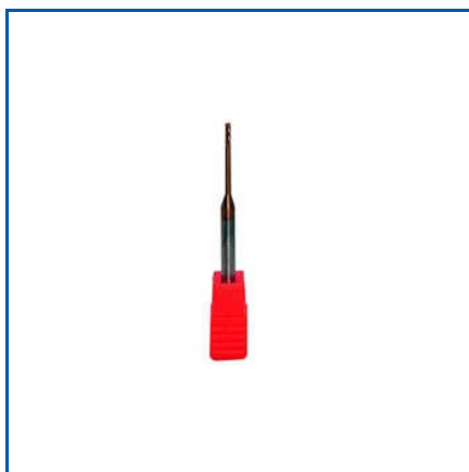
LN 1.5X16X50 4FLUTE BALLNOSE COPPER 55HRC TiCN COATED
