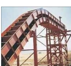
Bagasse Handling System
