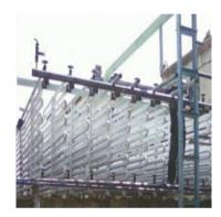
Atmospheric type Condenser Fabricated from 50NB MS C Class Heavy Duty Black Pipes with GI sprinkling arrangement Working Pressure 13 – 15 Kg cm2, Test Pressure 21 Kg cm2, Also we offer these coils with 100 micron Galvanizing to to prevent the corrosion from the water also it increases the life of condenser coil.
