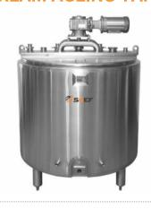
Type: Dimple jacketed, insulated vertical Tank Material: a) Inner shell-AISI 304 b) Intermediate shell - AISI 304 c) Outer Cladding - AISI 202 Finish: 150 grit Accessories: Inlet/outlet, temperature sensor, manhole, Agitator (top mounted) and other standard accessories.
