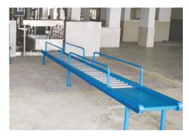
Roller conveyor will be fabricated out of Mild Steel C-channel or SS304 Square Box as per requirement & rollers made of 51 mm MS/SS heavy duty pipe provided with brass bush bearings/roller bearings for smooth rolling operation. The frame shall be supported on MS/SS legs fitted with ball feet 50m.
