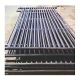
IBT ASTRA Design IBT Cooling Coils 6 mtr Length or as per tank size and Capacity Fabricated from 32NB MS C-Class Heavy Duty Black Pipes with Proper Header Arrangement at both end, Coils are tested with Hydro Pressure at 25 Kg/Cm2, Anti Rust Paint for Coils or Hot dip galvanizing can be done as per requirement.
