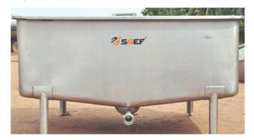
Rectangular, un-insulated from 300L-2000L capacity single as well as double compartment. The tank would be constructed from SS 304 sheets/coils, with slope towards outlet. The tank will be single compartment, complete with three pieces SS 304 covers with handles. The tank will be on SS 304 pipe legs with ball feet. The bottom outlet will be with a valve.
