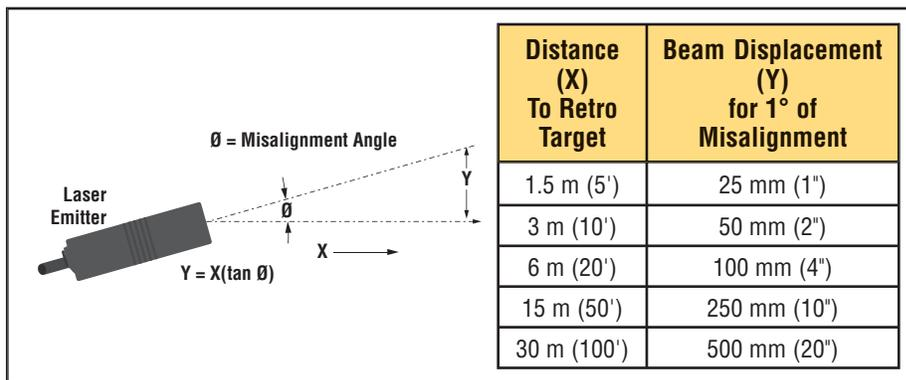
Figure 3. Beam displacement per degree of misalignment
