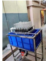
Plastic Goli Soda Bottle Rinsing Machine
