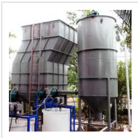
Lamella Clarifier System
