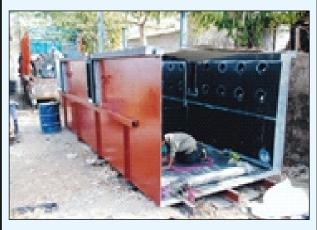
medium of application, pH value, temperature, abrasive nature e.g. Butyle, E.P.D.M., Polychloroprene, N.B.R., Hyplone, etc. We will mutually select the type of Rubber and the thickness of lining best suited for your operations and carryout the work as per the provisions of IS.
