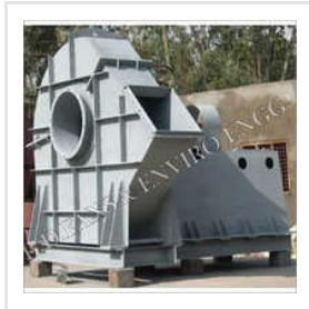
Induced Draft Fan
