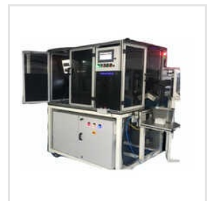
Automated Inspection And Sorting Station
