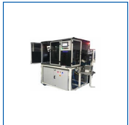
AUTOMATED INSPECTION AND SORTING STATION
