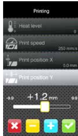
Print position Y Fast setup with a slider, fine setup with \pm keys
