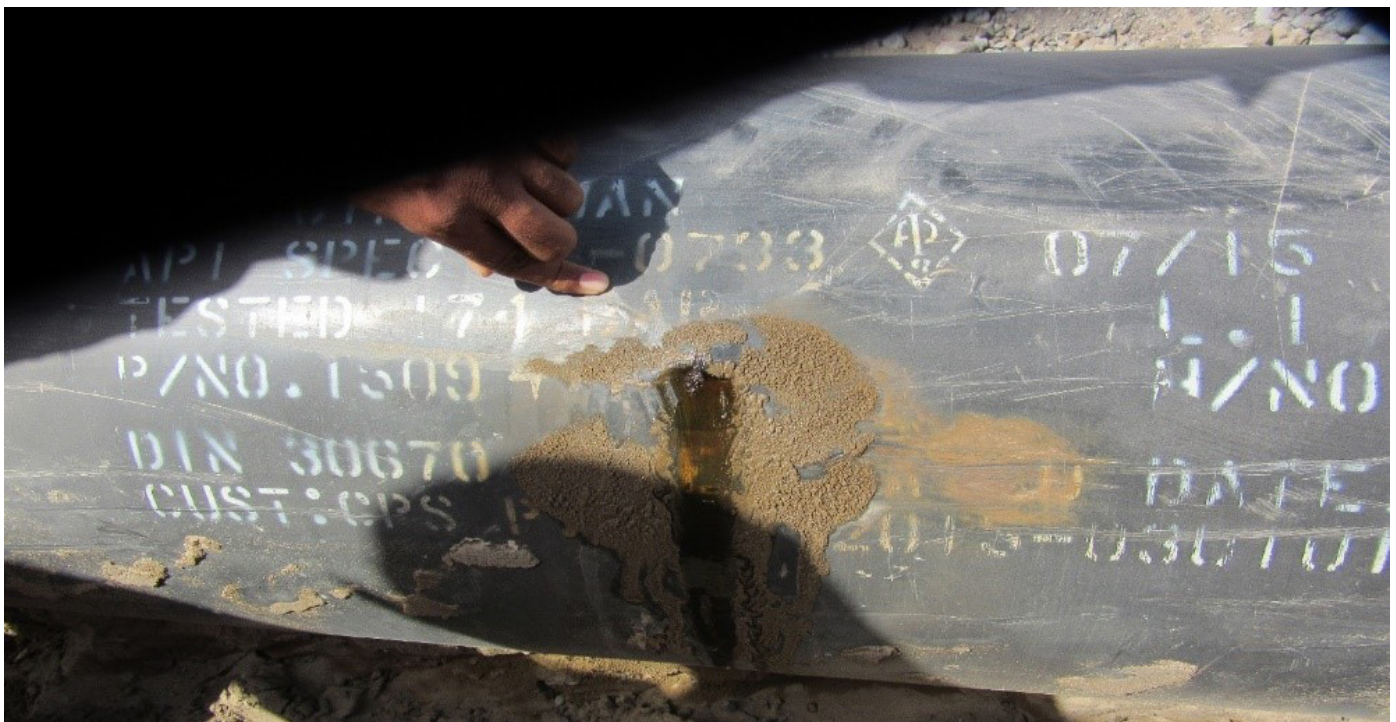
Figure 5: Leak detected on a pipeline in Oman using the Pig Point technique
