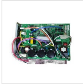
Toshiba Inverter AC Printed Circuit Board
