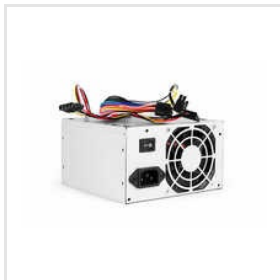
Electric Power Supply Unit
