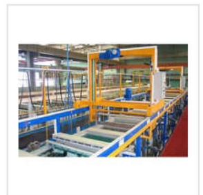
Fully Automatic Electroplating Plant
