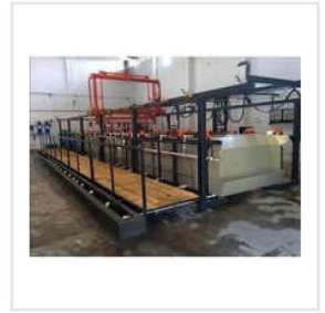
Transporter Wagon Electroplating Plant
