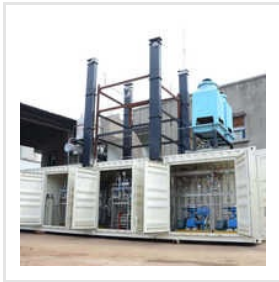
Industrial Hydrogen Generator
