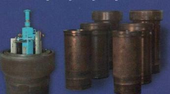
Cracked parts need only be dismantled in exceptional cases. As the repairs are carried in cold process, no distortion or thermal stress is induced. Metal Stitching "locks", master-locks" and "plugs" are imported from U.K.
