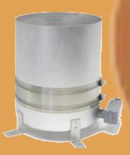
Kaizen make snow water Equivalent recorder is a self contained fully automatic SWE data recorder fitted with solar panel & SLA battery based power system, High accuracy Vlog data logger & power managment system contained in a single IP65 waterproof enclosure.
