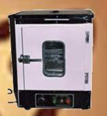
Temperature range up to 90 Degree C. Heating elements are placed in ribs on all the three sides. Doubled walled inner chamber made of anodized S. Steel. Outer chamber of M. Steel duly painted. Door has double glass window to view samples.
