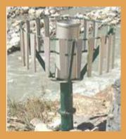
There is great variety of snow gauge available. The one we offering is of mechanical type used in measuring stick inside a metal jar and core to the earth. This works well for the measurement of Snow Water Equivalent. Accurately measures fallen snow depths up to 30".the product has lost lasting components, easy
