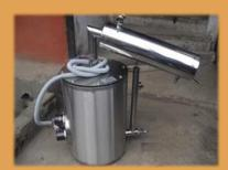
Its double walled the outer is made of M.Steel painted with white stoving enamel and inner (Boiler) is made of S.Steel. The gap between walls is filled with special grade glass wool to avoid lots of
