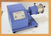
For mixing and grinding electricity operated. Having capacity up to 1 kg fitted with FHP geared motor with maximum speed of 80 RPM. Jar is made of
