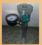
soil, it will allow water to flow freely through it, but not air. Tensiometer is available in standard lengths of 15, 30, 45, 60, 90, 120 cm. General use with row, tree, and field crops. Includes reservoir, air free gauge chamber, and hermetically sealed dial type vacuum gauge with dual
