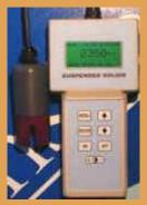
It is a unique system that combines advanced electronics with a solidstate, optical sensor. It is a multi range indicator designed for the measurements of suspended solids in aqueous solution. The microprocessorbased electronic of the indicator provide a high degree of flexibility and
