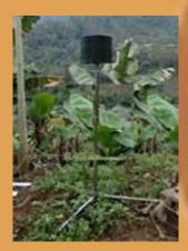
The Digital Rain Gauge With In Built Data Logger we offering shows the Operating temperatu range from -20°C to 70°C, Time accuracy: ±1 minute per month at 25°C, Battery life: one year typical use, Sensors inbuilt are Tipping Bucket Rain Gauge With Read Switch, Resolution and Accuracy: 0.20 mm with 5% up to 100mm / hour and more.
