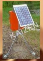
Automatic soil moisture suction & Soil Temperature Recorder is a complete system for monitoring, logging and graphing 7 point Soil moisture & 1 point soil Temperature readings. Automatically reads the sensors, 12v battery powered monitor, battery Charging through Solar Panels, Reading frequency from every minute to every day and adjustable to suit you, 8 sensor
