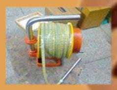
Export Quality water level indicator is a trustworthy instrument for measuring the level of water and total deepness in boreholes, well, reservoirs etc. for the measurement the bob is lowered to the water level. When
