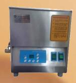
Outer is made of stainless steel. OPERATING FREQUENCY: 36 +/- 3 KHz or 22 +/- 3 KHz Maximum Temperature Range: 700 C Resolution: 10C Accuracy: +/-20C Sensor: PT - 100 RTD Sensors
