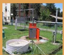
Kaizen make Digital Solar Radition Recorder is a self contained fully automatic solar data recorder fitted with solar panel & SLA battery based power system, High accuracy V-Log Data Logger & Power managment system contained in a single IP65 waterproof fenclouser.
