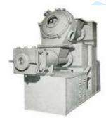
The plodder is commonly used by Soap manufacturing units is a very important equipment which is specially designed with heavy duty gear train, breakearms and load thrust carrier. It plods the mass of material and extrudes the soap or detergent particular shape or design of the soap bar Die is provided on the plodder.
