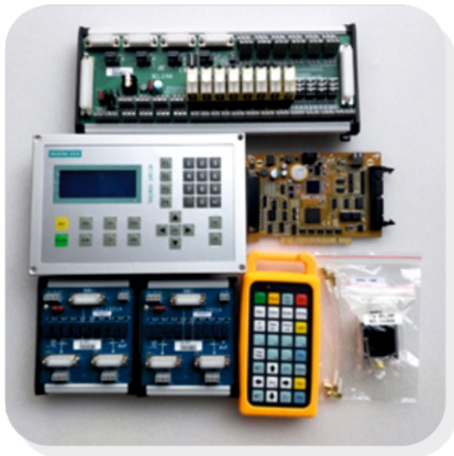
Control System (Cypcut/Raytool)
