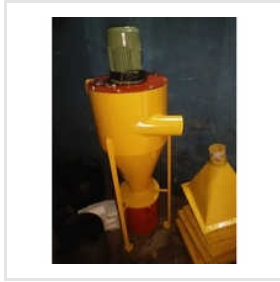
Flour Mill Dust Collector
