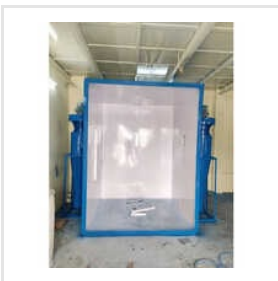
Dust Control Booth
