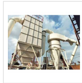
Automatic Dust Collector
