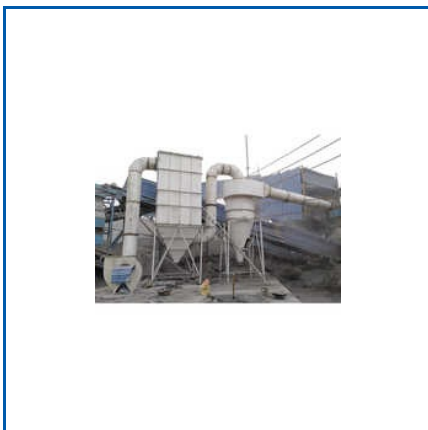
PULSE JET DUST COLLECTOR SYSTEM
