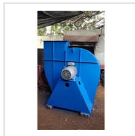
Industrial Centrifugal Blower
