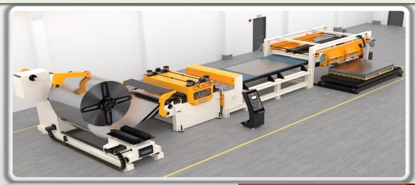
SRE cut-to-length lines (CTL) can be used to process hot-rolled and cold-rolled galvanized, pre-painted and stainless steel coils, as well as non-ferrous materials - aluminum, copper and brass coils. Process metal coils by uncoiling, straightening, cutting to length and stacking metal slabs. These lines offer automation to ensure accurate feeding, flattening and shearing for a variety of industries.
