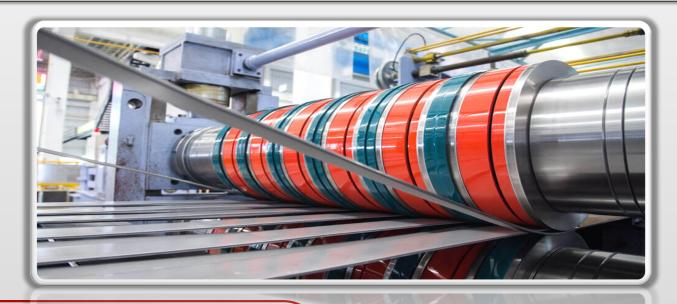
This equipment is a special shearing equipment for processing steel coils into narrow strips required by customers by uncoiling, slitting and coiling. It is mainly composed of uncoiler, pinching and straightener, slitter, tension machine, coiler, etc., and is supplemented by feeding, side guiding, transition and conveying sections.
