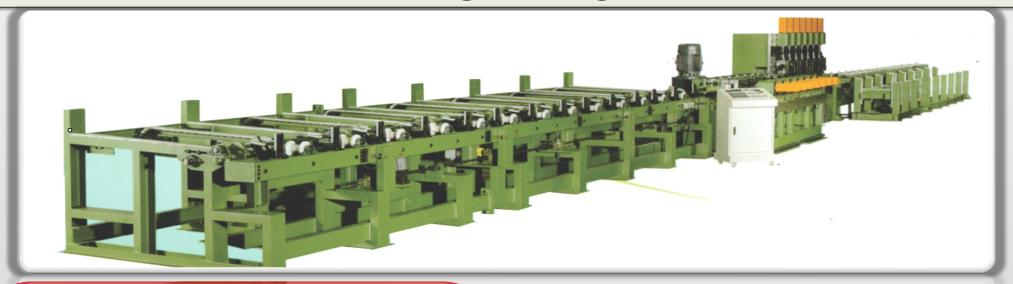
The roller type section straightening machine is most suitable for straightening of any rolled drawn or extruded ferrous and non-ferrous section in cold condition. This machine is engineered to give trouble free long life service. The body and base are fabricate form mild steel plates duly stress relieved and machine as per design. All straightening rolls (top and bottom) are mounted on cantilever type spindle. This arrangement is most suitable where quick change of rolls are required.
