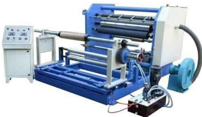
Center Shaft Slitting Rewinding Machine
