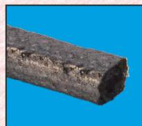
A 100% pure GRAPHITE YARN packing impregnated with a Blocking Agent. GRAPHITE fibers do not harden or glaze at high temperature. With lubricating value of graphite, the packing is frictionless eliminating shaft wear. The packing has high heat conductivity, high temperature resistance and low co-efficient of expansion.
