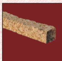
Basically this Non-Asbestos packing is for Marine Stern GLANDS. Manufactured from long life natural flax fiber yarn impregnated with PTFE and additional lubricant, specially blended for hydraulic applications, combining strength, firmness, flexibility, lubricity and compressibility.
