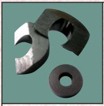
CHAMPION STYLE 660 is a high purity (99.00% to 99.9% carbon), self lubricating and anti-frictional die molded, pre-formed gland packing ring manufactured from Flexible Pure Graphite Foil. These rings are manufactured in endless form or in 2 halves in oblique cut containing no oil or grease binder / additive of any kind.
