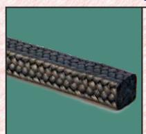
Champion Style 6100 is a synthetic fiber based packing with adequate lubrication of a proprietary special graphite dispersion which simultaneously impregnates the packing to give leak free service and also acts as a lubricant to ensure smooth running of the pump, without scoring of the shaft.
