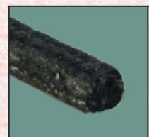
Champion Style 7916 is an asbestos replacement. Champion Style 7916 is a lubricated ceramic kiln seal packing reinforced with metal wire with superior seal ability. This is an ideal choice for high temperature valve applications and is extremely suitable for high temperature & high pressure service conditions, handling temperatures ranging from -50°C to +1250°C.
