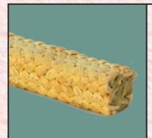
This Abrasion resistant, inert packing is produced from tough high strength ARAMID fiber filament yarn with each strand fully impregnated with PTFE high temperature resisting lubricants. The packing has flexibility, resiliency, lubricity with excellent thermal and dimensional stability, treating the shaft gently.
