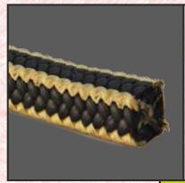
A combination of tough ARAMID fiber yarn in the corner and core strands and PTFE GRAPHITE yarn on the seam strands. This structure generates maximum resistance to extrusion; simultaneously the graphite PTFE yarn on the sides of the packing imparts thermal conductivity and lubricity for cooler shaft running.
