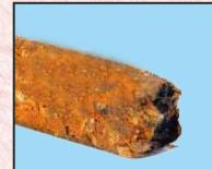
The packing is made from longline natural flax fiber yarn, in square braided construction having combining strength, flexibility & compressibility. The yarn is thoroughly impregnated during the construction process with a non graphite lubricant and further surface treated with a special water resistant lubricant.
