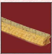
CHAMPION Style 175 is a unique packing specifically manufactured for abrasive media. This packing is manufactured from a special polymer highly resistant to abrasion. The packing is incorporated with high anti-frictional and inert fluoro polymer lubricants which makes the packing very soft but compact and firm. By incorporating a select run-in-lubricant, the packing becomes highly resilient.
