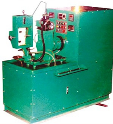
Conventional jar-type fuel injection pump test stand.
