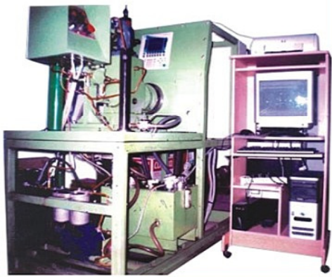
Computerised fuel injection pump test stand for ALCO locomotives.
