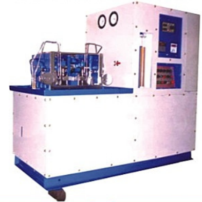
Unit injector test stand, model S-GM2, for testing GM-EMD 710 series loco engine mechanical unit injectors.
